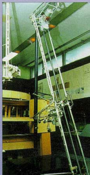
"Луна" с ГЗУ, испытанные в BK600/300. with the ground-catching device tested in the chamber VK600/300
